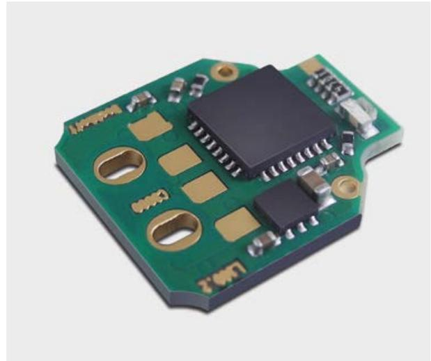
Precise cuts for depaneling PCBs, drilled round holes, or nonround apertures can be achieved by the laser in a single processing step (source: Smyczek GmbH).
