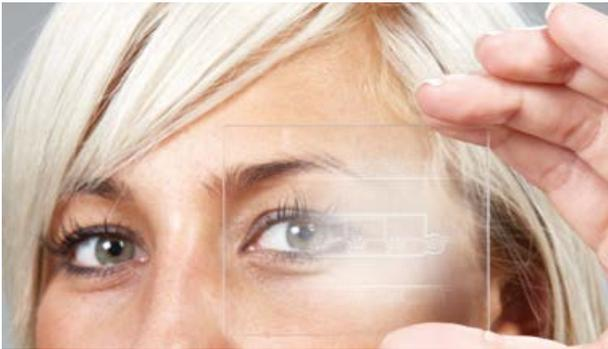
Breathing on the glass plate reveals the previously invisible conductive TCO layers
